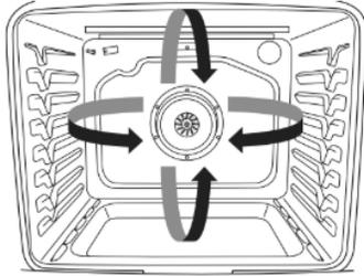
During convection cooking, the bake, broil, and convection elements cycle on and off in intervals to maintain the oven temperature, while the fan circulates the hot air.
