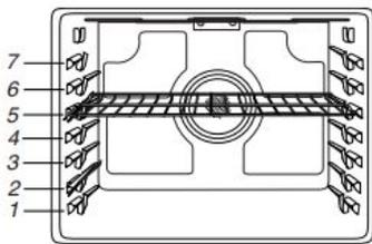
The oven has 7 positions for a flat rack, as shown in the previous illustration and the following table.
